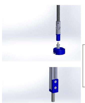
Screw the clamp in the aluminum bush for at least 5 mm, find the desired position and tighten nut + washer to lock the rotation.
