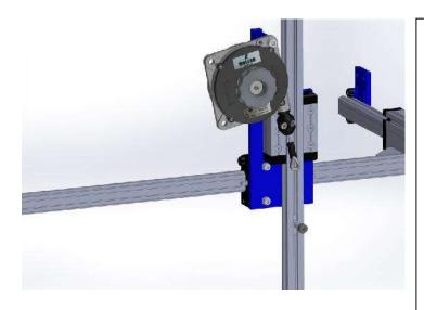
Loosen the screw, insert it in the loop of the balancer and screw it into the nut inside the rail.
