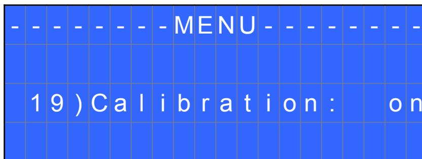
3. Press OK to confirm. If you choose OFF, calibration will be interrupted and no torque value will be displayed. You choose ON, calibration will continue and the following screen will be displayed:
