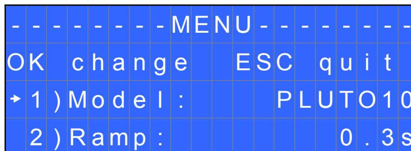
**1) Model:** you can select the screwdriver to be used. Your choice will automatically change the default settings. It's important to select the correct model you're going to use since many parameters regarding the motor software are specific for every single model.
