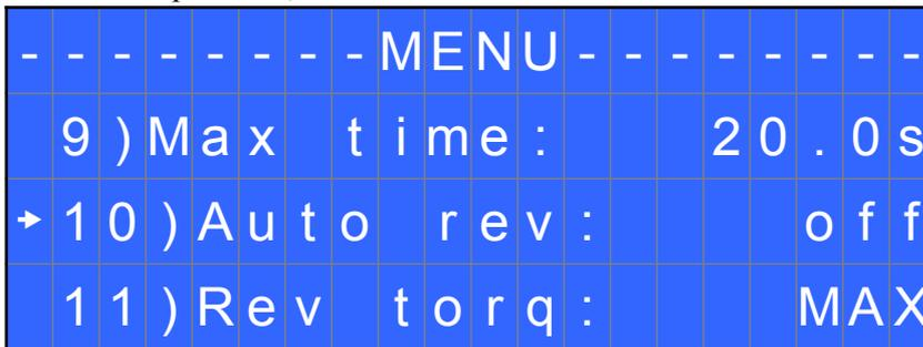
**9) Max time - Maximum time:** You can select the maximum time of tightening. You can set from 'Min time + 0.1s' to 20.0 sec.
