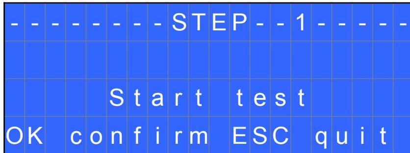
Complete a screwing cycle on the mini k5 and take note of torque value.
