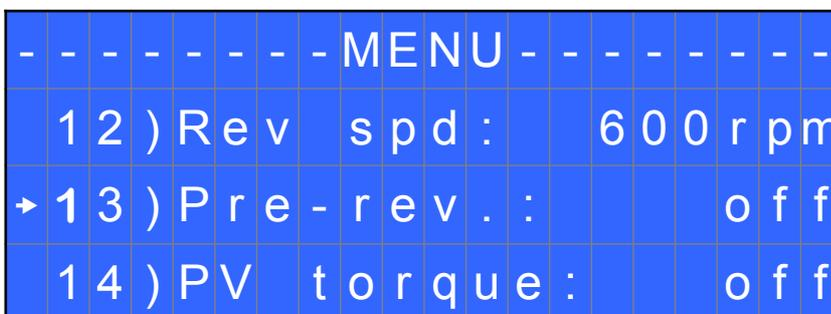
**12) Rev speed – Reverse speed:** You can select any reverse speed value of the screwdriver between the maximum and the minimum specific speed of every single screwdriver (see table with technical data).
