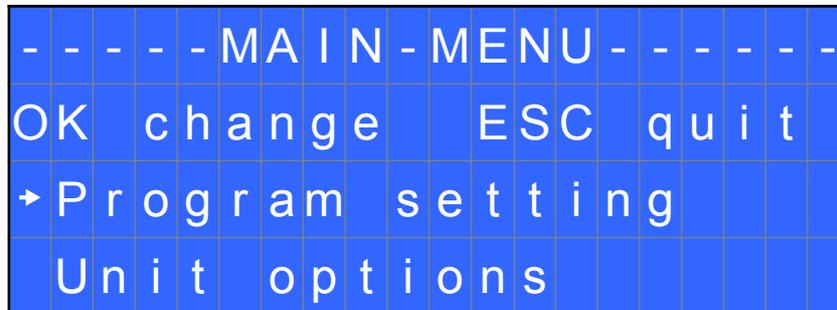
**Program setting:** It indicates the menu section where you can set or modify the fastening parameters.
