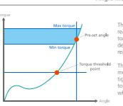
This mode gives priority to the angle to be reached. Starting from the pre-set threshold torque, the system will start counting the degrees and when the pre-set angle is reached the screwdriver will stop.
